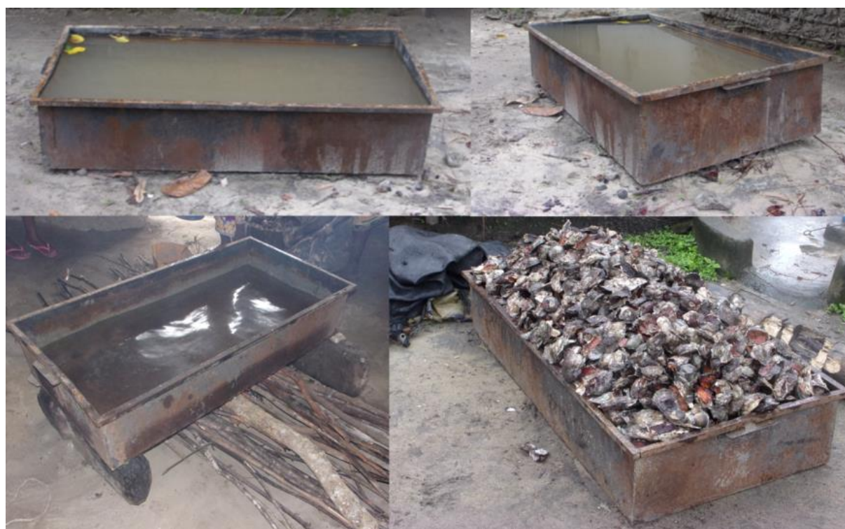
Plates 1a-d. Up-scaled steaming troughs rolled out during the 2018 Bonthe Oyster festival
